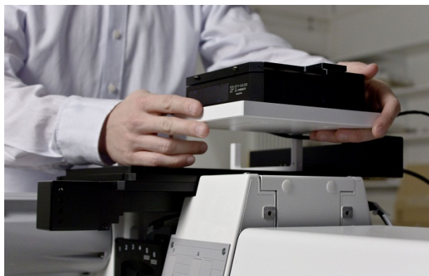
Fig. 6 The fine adjustment of object or sample is carried out by the piezo nanopositioning system, which not only operates with high accuracy but can also be readily integrated into the application (Image: PI / Nanoscribe GmbH)
